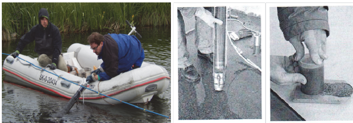
Obr. 4. Odber nánosov pomocou beekera (vľavo) a detail vzorky nánosu (vpravo). Fig. 4. Extraction of silt material using beeker (left) and detail of silt sample (right).
