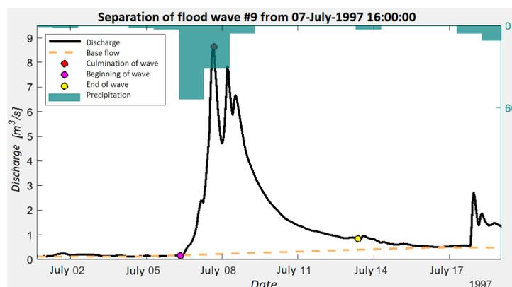
Fig. 1. Example of a flood wave separation in the FloodSep programme (Valent, 2019).
