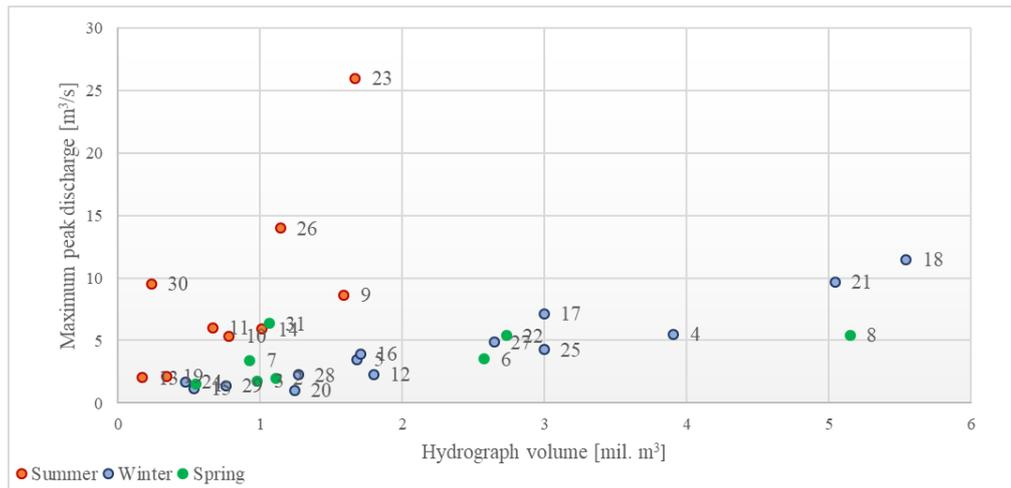
Fig. 5. Relationship between a flood's volume and peak discharge – annual maximum discharges.
