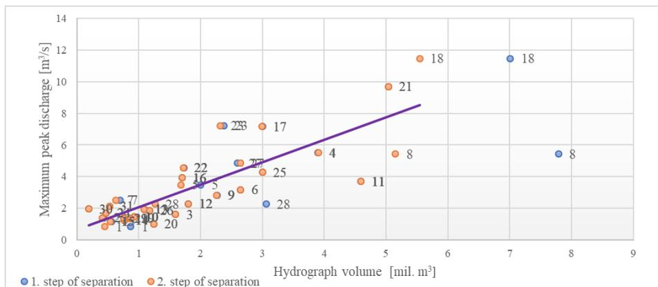
Fig. 4. Relationship between a flood's volume and peak discharge: results of discharge-wave separation in the Winter season.
