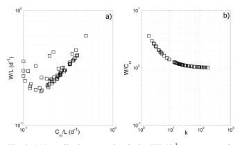
**Fig. 6.** a) Normalized wave peak velocity W/L (d<sup>-1</sup>) versus normalized celerity  $C_a/L$  (d<sup>-1</sup>) vs. b) ratio between wave peak velocity and celerity  $W/C_{\omega}$  versus hydraulic Peclet number k.
