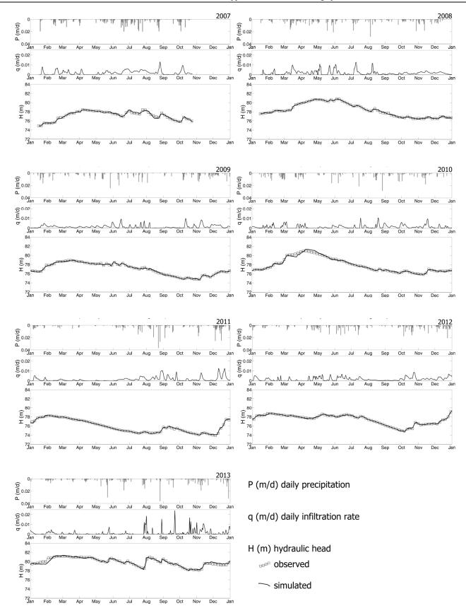
Fig. 3. Daily precipitation P (m/d), daily specific infiltration flow rate q (m/d) that reaches the water table and simulated and observed hydraulic heads H (m) for the period 2007–2013.
