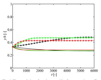
**Fig. 4.** Time evolution of gravity centroids of concentration profile of  $c_A$  and  $c_B$ , for  $r_A = r_B$ ,  $m_A = m_B$ , for 3 different flow slopes as in Figure 3. Legend: increasing curves with symbols = fraction B, decreasing curves = fraction A (black -  $\phi = 20^\circ$ , green -  $\phi = 26^\circ$ , red -  $\phi = 30^\circ$ ).
