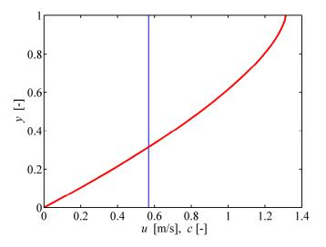
**Fig. 1.** Velocity profile (using Eq. (13)) and total concentration profile for e = 0.65,  $c_M = 0.586$ ,  $r_B = 1.1r_A$ ,  $\phi = 25^\circ$ . Legend: red line - velocity profile, blue line - total concentration profile for mixture of two fractions.
