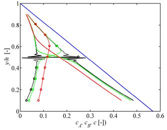
**Fig. 3.** Final concentration profiles of  $c_A$  and  $c_B$ , for  $r_A = r_B$ ,  $m_A = m_B$ , at dimensionless time 6000 for 3 different flow slopes. Legend: inclined blue line – total concentration, lines with symbols – spheres A, lines without symbols - spheres B (black -  $\phi = 20^\circ$ , green -  $\phi = 26^\circ$ , red -  $\phi = 30^\circ$ ).
