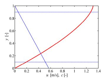
**Fig. 2.** Initial profiles of velocity and total concentration. Legend: red line – velocity profile, inclined blue line – concentration profile, horizontal blue lines – range of computation.
