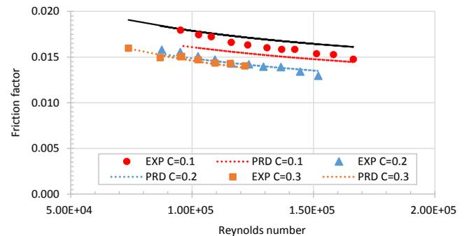
**Fig. 4.** Predicted versus measured friction factor  $\lambda_m$  in 0.026 m pipe for sand slurry;  $d_{50} = 1.5$  mm;  $\rho_p = 2650$  kg/m<sup>3</sup>.
