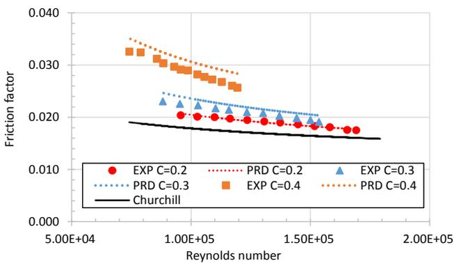
**Fig. 6.** Predicted versus measured friction factor in 0.026 m pipe for coarse PVC slurry;  $d_{50} = 3.4$  mm;  $\rho_P = 1400$  kg/m<sup>3</sup>.
