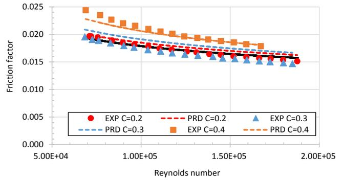
**Fig. 2.** Predicted versus measured friction factor  $\lambda_m$  in 0.026 m pipe for polystyrene slurry;  $d_{50} = 1.5$  mm;  $\rho_p = 1045$  kg/m<sup>3</sup>.
