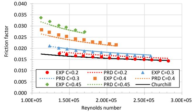
**Fig. 7.** Predicted versus measured friction factor in 0.04 m pipe for coarse polystyrene slurry;  $d_{50} = 2.8$  mm;  $\rho_P = 1045$  kg/m<sup>3</sup>.
