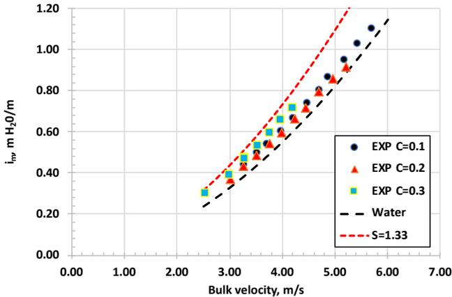
**Fig. 9.** Measured frictional head loss for slurry flow. Sand particles:  $d_{50} = 1.5$  mm,  $\rho_P = 2650$  kg/m<sup>3</sup>, pipe diameter  $D = 0.26$  mm (Bartosik, 2009).
