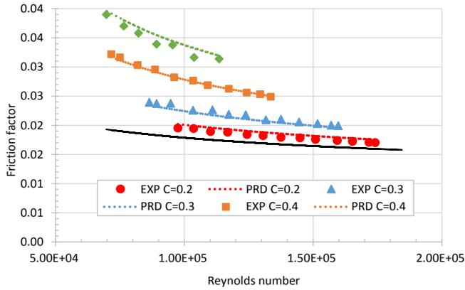
**Fig. 5.** Predicted versus measured friction factor in 0.026 m pipe for coarse polystyrene slurry;  $d_{50} = 2.8$  mm;  $\rho_P = 1045$  kg/m<sup>3</sup>.
