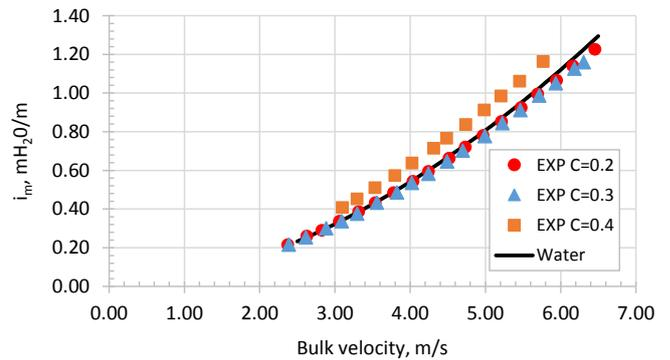
**Fig. 3.** Measured frictional head loss for slurry flow. Polystyrene particles:  $d_{50} = 1.5$  mm,  $\rho_p = 1045$  kg/m<sup>3</sup>, pipe diameter  $D = 0.26$  mm (Shook and Bartosik, 1994).
