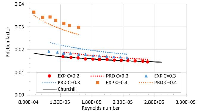
**Fig. 8.** Predicted versus measured friction factor in 0.04 m pipe for coarse PVC slurry;  $d_{50} = 3.4$  mm;  $\rho_P = 1400$  kg/m<sup>3</sup>.
