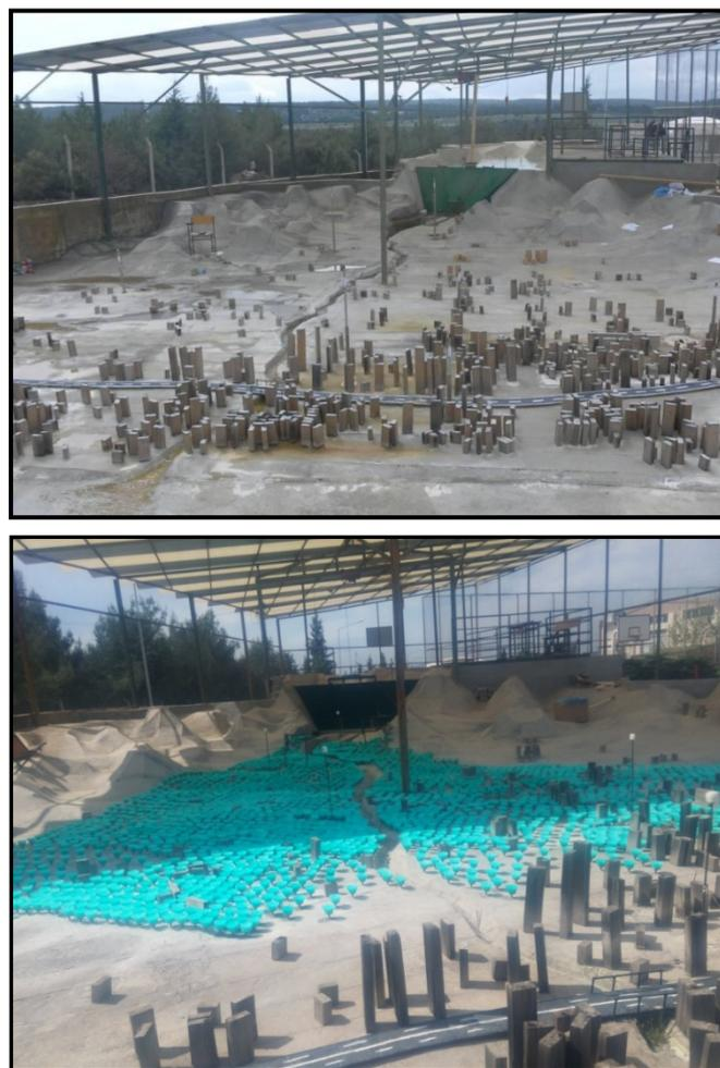
**Fig. 1.** Physical model of Urkmez Dam Lake and downstream region without vegetation and with vegetation.
