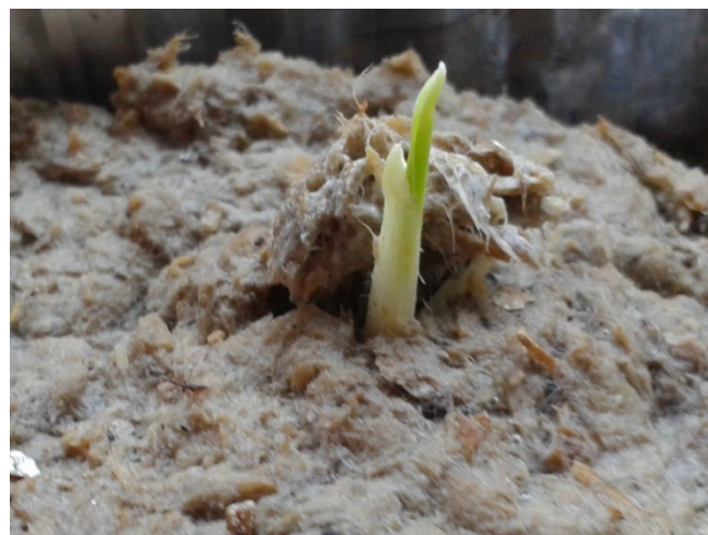
Fig. 1. Sprout of Sorghum halepense that had passed through a wet layer of the prototype hydromulch by punching it.
