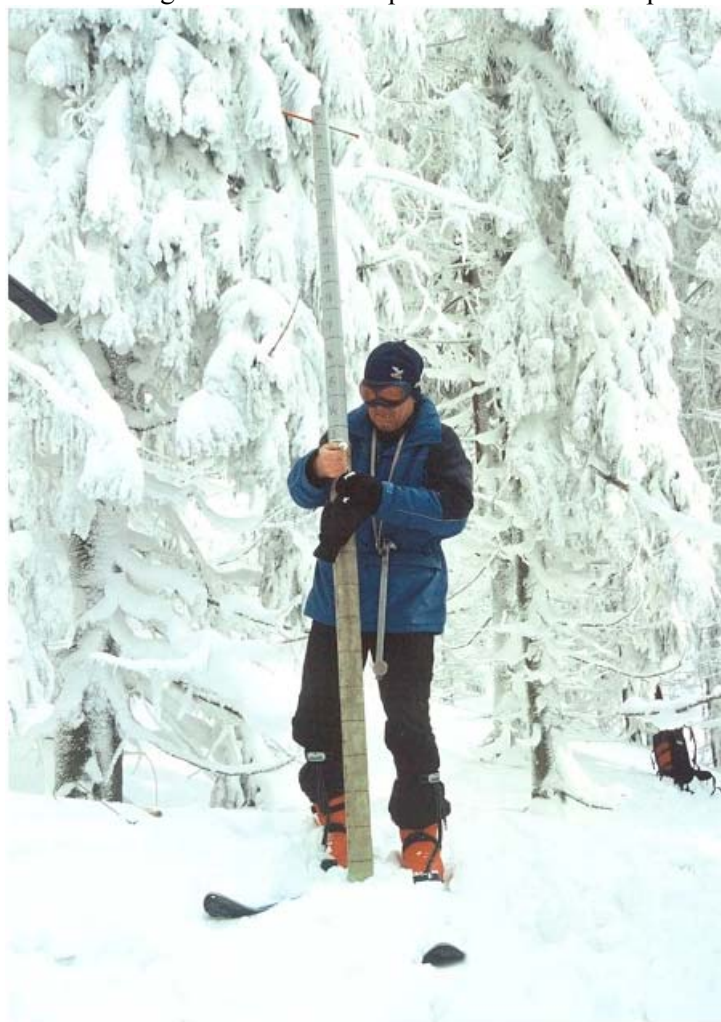
Obr. 3. Nadstavená snehomerná rúra pre použitie v hlbokom snehu. Fig. 3. Adjustment of the length of snow sampler for measurement in deep snow.
