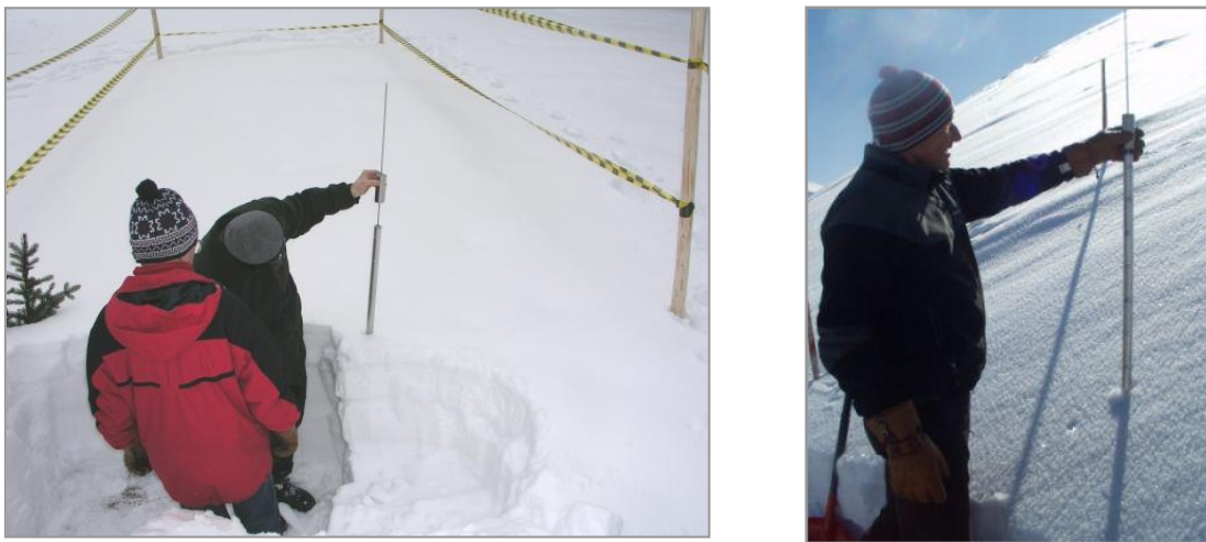
Fig. 2 Sounding by stamping
