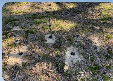
Figure 4. Field measurements with minidisk infiltrometer.
